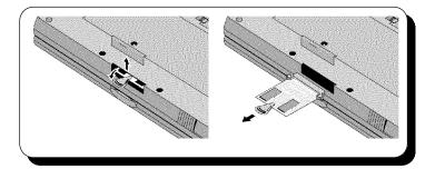
To install a RAM module, use the reverse procedure. Make sure that the pull tab is on the bottom.
