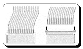
Slide the sleeves of the keyboard connectors forward and remove the cables (see illustration to the left for removal of cables). A small probe will help get to the sleeves and in alignment of the cable during installation.
